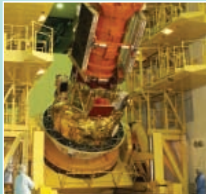
The Fregat Upper Stage of the Soyuz Rocket with all payloads fully integrated onto it. The huge orange coated satellite is the Meteor M-1 and SumbandilaSat is the tiny black square on the left.
